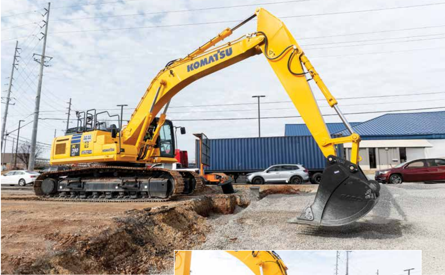
An operator lays gravel to grade and smooths the surface with a Komatsu PC390LCi-11 IMC excavator.
