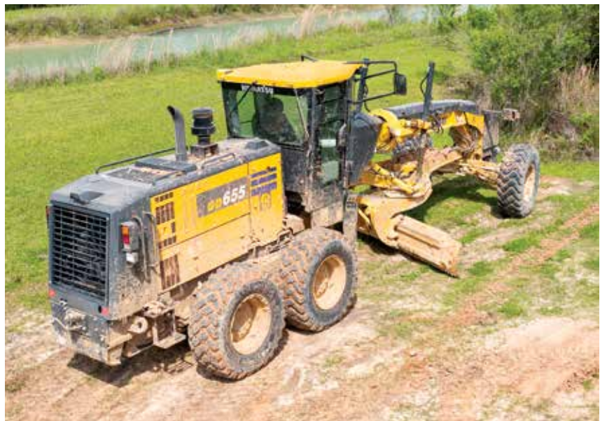
Oil-Dri uses a Komatsu GD655-7 motor grader to maintain its haul roads.
