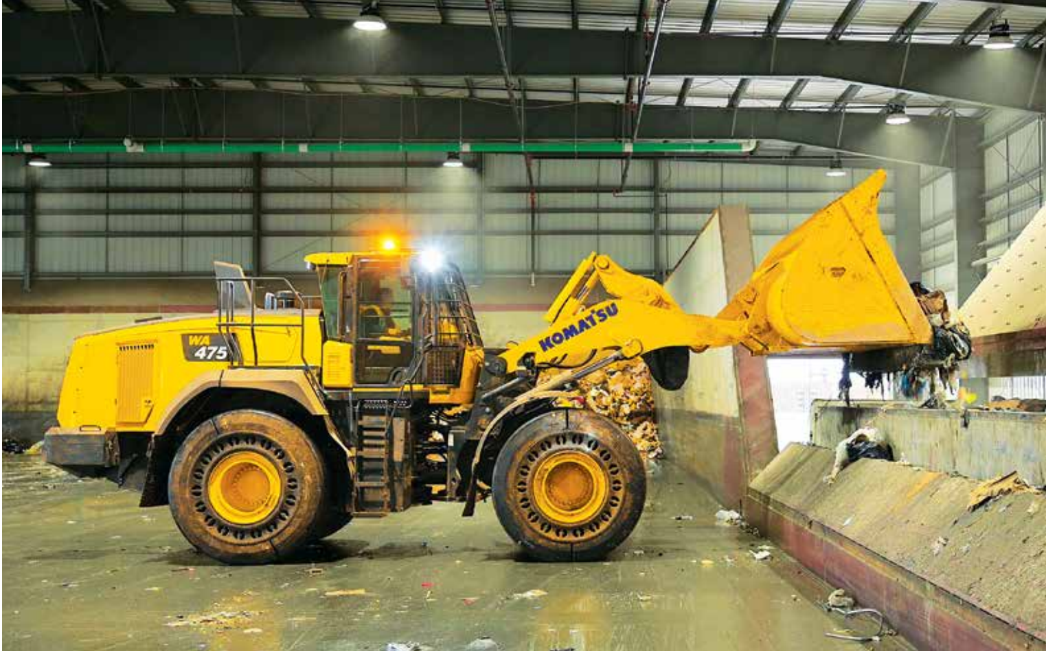
The Komatsu WA475-10 WH wheel loader features guarding on the bucket cylinder, front and rear frame, axle seals, fuel tank, articulation point and a boom cylinder hose.
