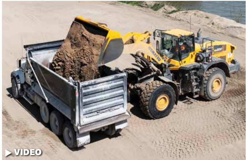
With a Komatsu WA500 wheel loader, an operator loads sand into a haul truck.
