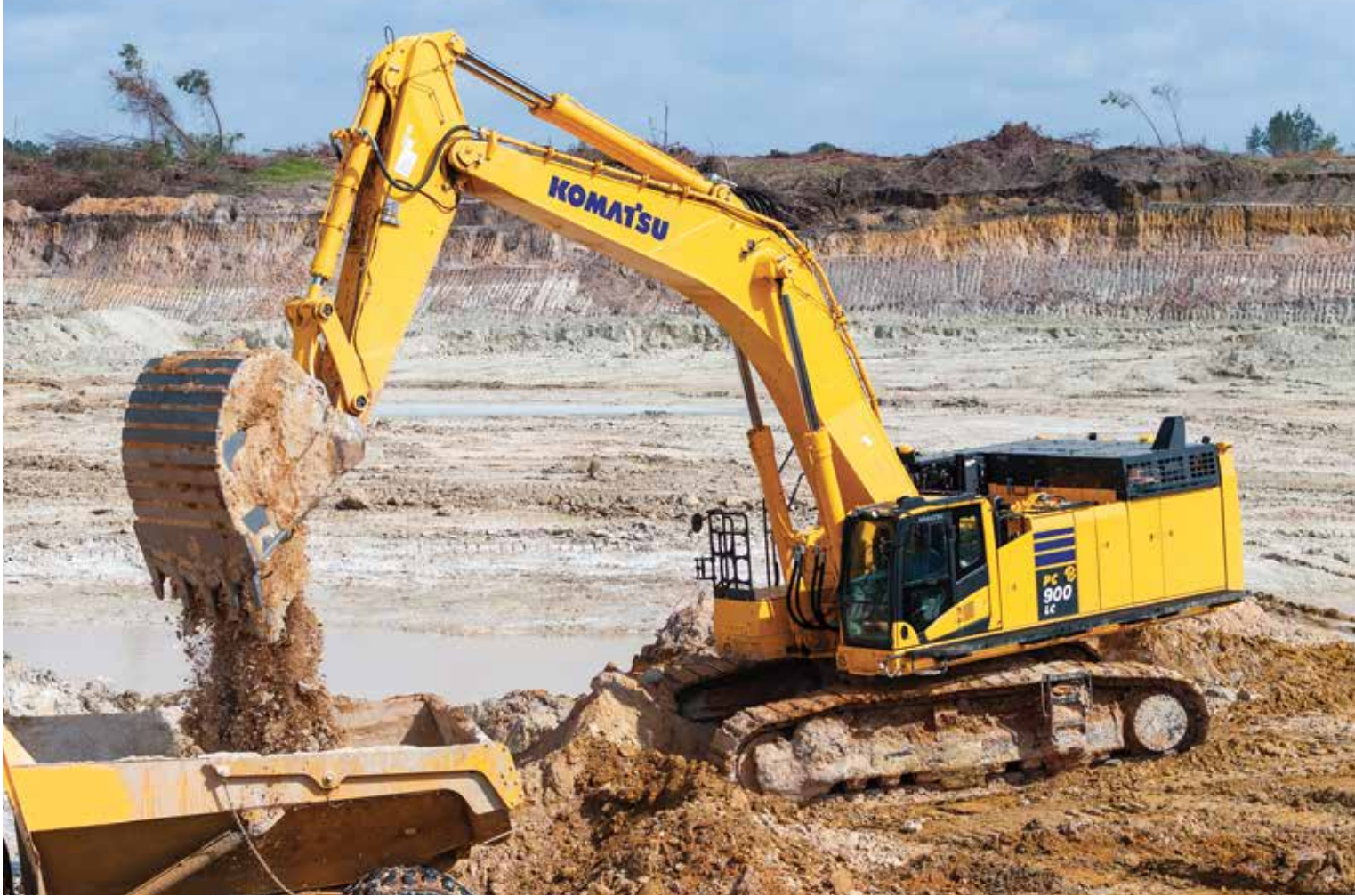
An operator loads a haul truck in three passes with a Komatsu PC900LC-11 excavator.
