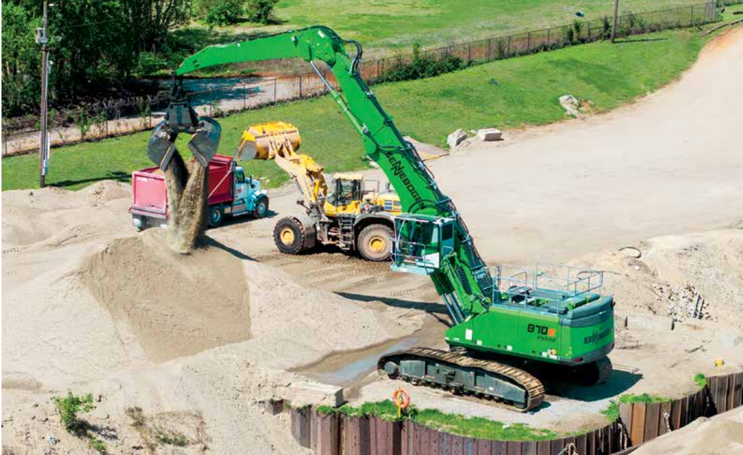
Operators work together using a Komatsu WA500 wheel loader and a Sennebogen 870 E hybrid material handler to unload sand from a barge, into a staging area, and then to a haul truck.
