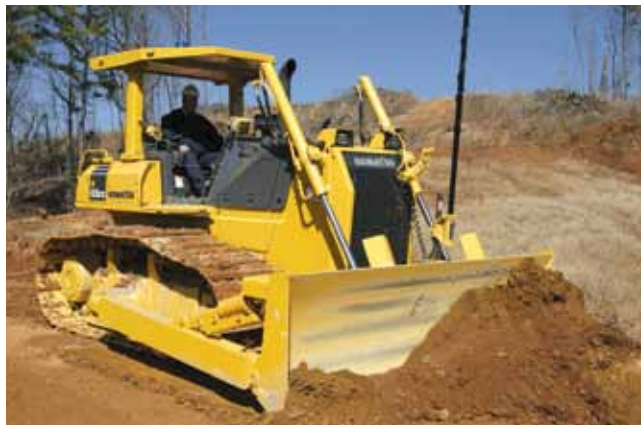
Komatsu has worked closely with laser-grading manufacturers to come up with a new 3-D machine-control system that dramatically improves fine dozer grading.
